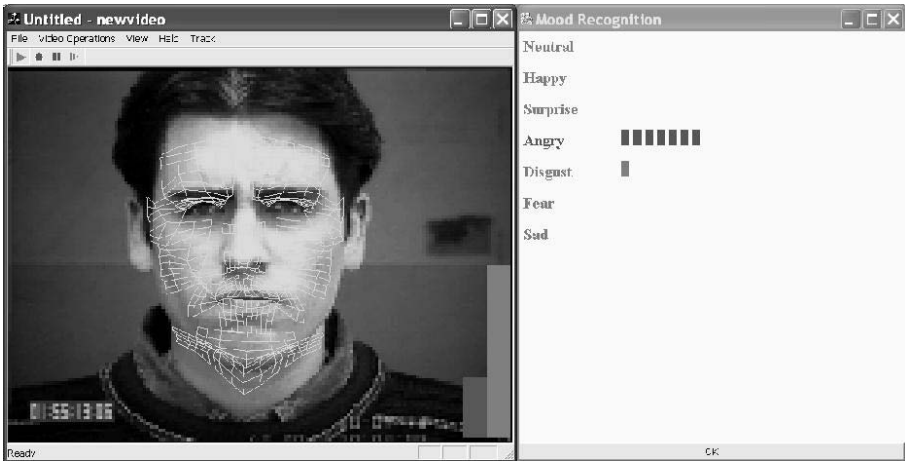
Figure 10.2. A snap shot of our realtime facial expression recognition system. On the right side is a wireframe model overlayed on a face being tracked. On the left side the correct expression, Angry, is detected (the bars show the relative probability of Angry compared to the other expressions). The subject shown is from the Cohn-Kanade database [Kanade et al., 2000].
